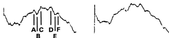
Fig. 5. PZNQR absorption curves used to estimate \eta for \text{KCu}(\text{CN})_2 .
