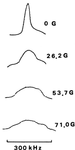
Fig. 6. PZNQR absorption curves of ^{75}\text{As} in \text{As}_2\text{O}_3 (arsenolite).
